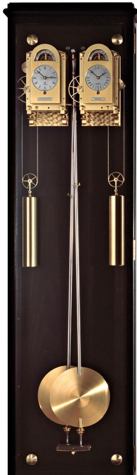
This double regulator is equipped with two identical and independent precision movements, each with a one-second pendulum. Shortly after setting both pendulums in motion, it will become noticeable that they settle into a mode seeing them swing in opposition; in other words, displaying a phase shift of 180 degrees.
