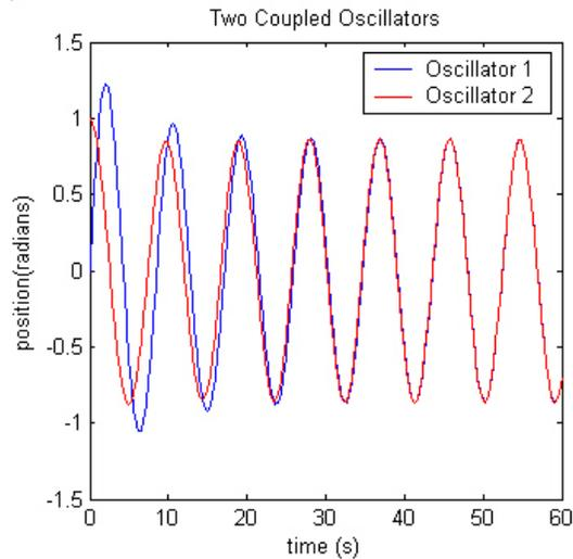
Figure 8: Coupled Oscillator Pair
