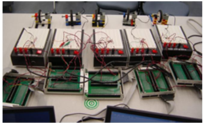
Figure 9: 5 Coupled Oscillators
