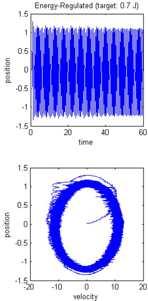
Figure 6: Energy-Regulated Damping
