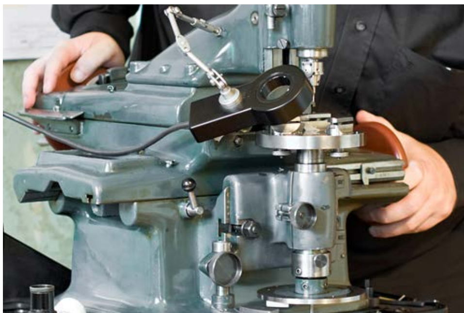
Beat demonstrating the use of the jig boring machine
