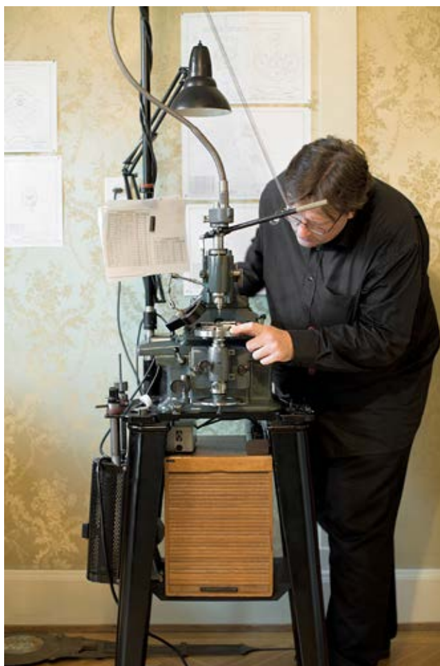
Another marvel: a jig boring machine dating from the thirties
