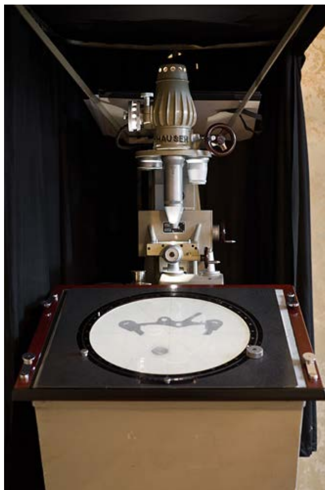
Elegant measurement apparatus magnifying a Haldimann lever
