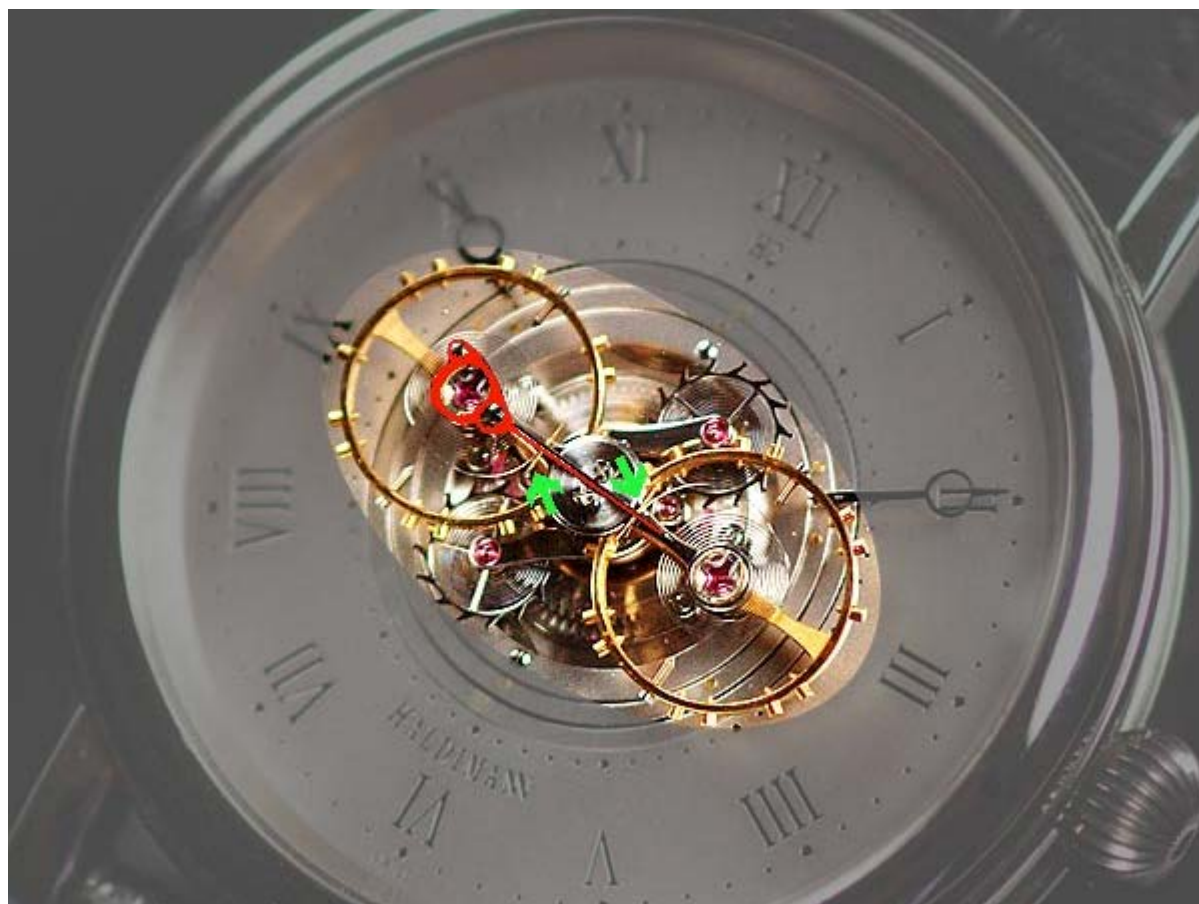
red:resonance coupling spring - green arrows: hairspring point of attachement
