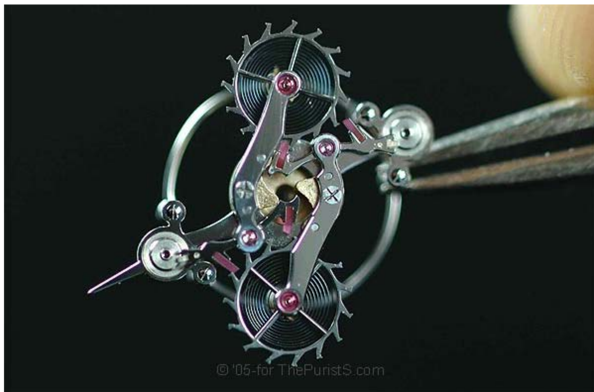
tourbillon carriage base with escape wheels and pallets note: the remontoire spiral springs concentric, below both escape wheels
